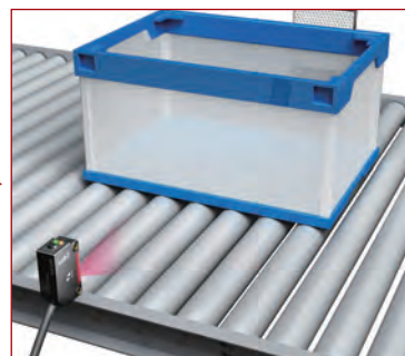
Target is now detected correctly. Note: Highly transparent objects cannot be detected. Check with actual target objects before running a machine.
